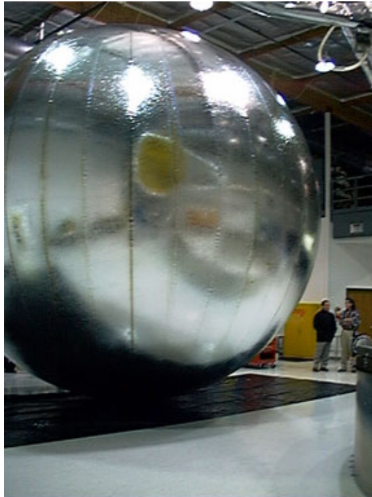
Figure 7. 1.75 m Radius Optical Calibration Sphere from L'Garde Inc., Launched January 6, 2000.
